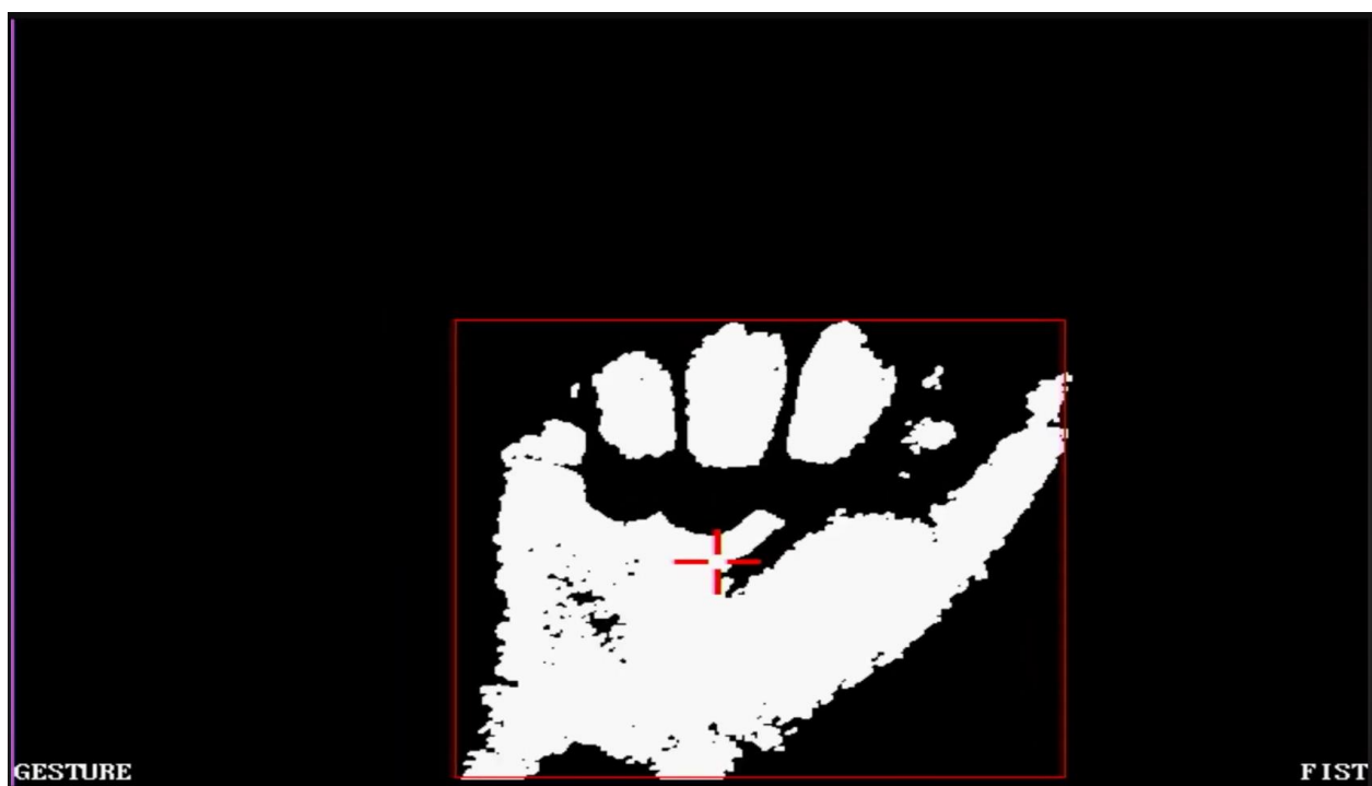
Figure 36: Gesture Recognition Video Output for Fist
