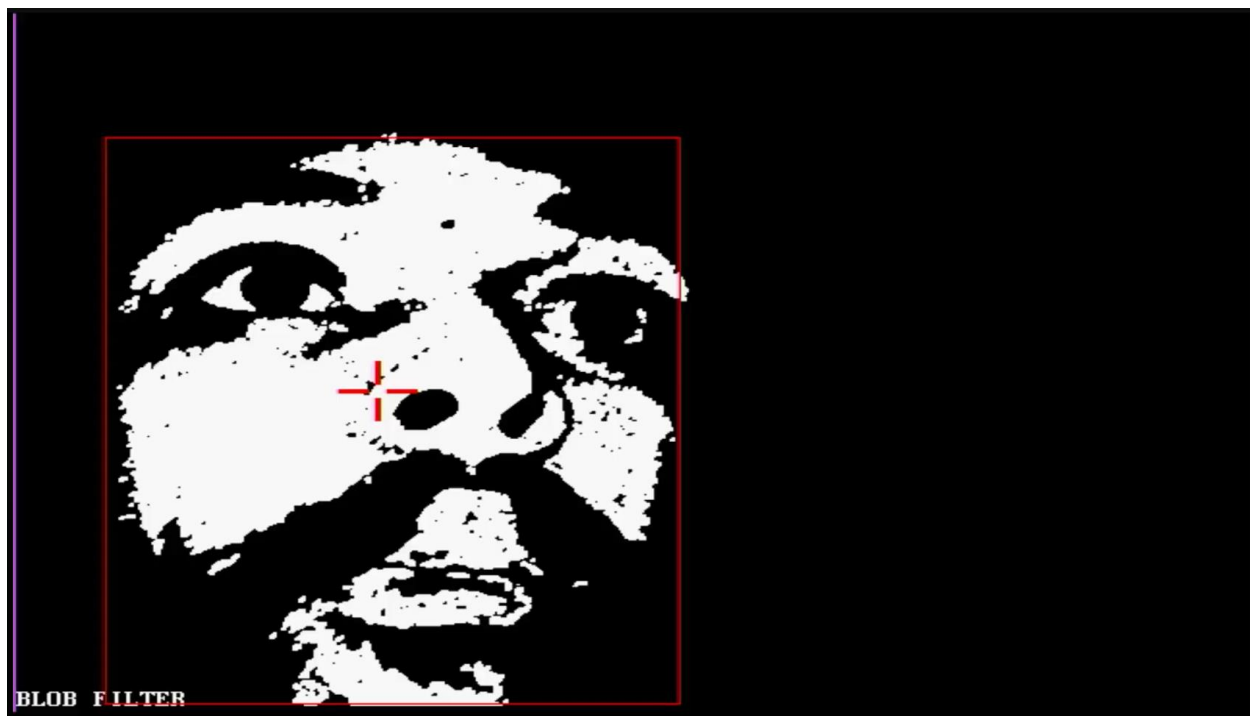
Figure 34: Blob Filter Video Output with Bounding Box Overlay
