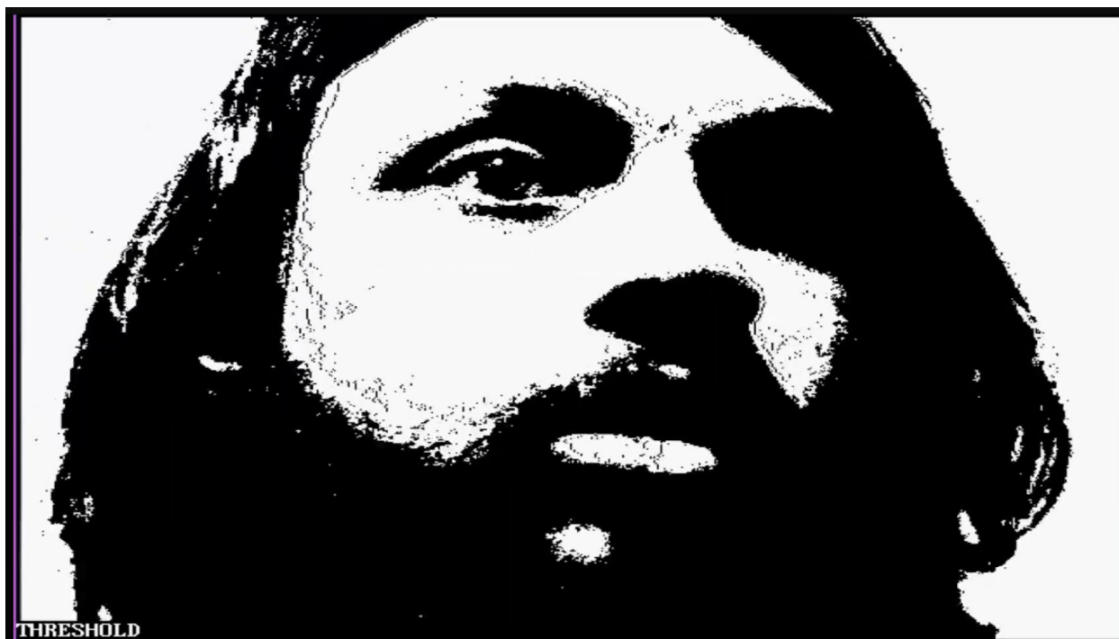
Figure 20: Thresholded Video Output
