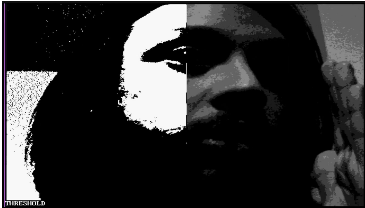
Figure 21: Thresholded Video Output with Split-Screen Grayscale Overlay
