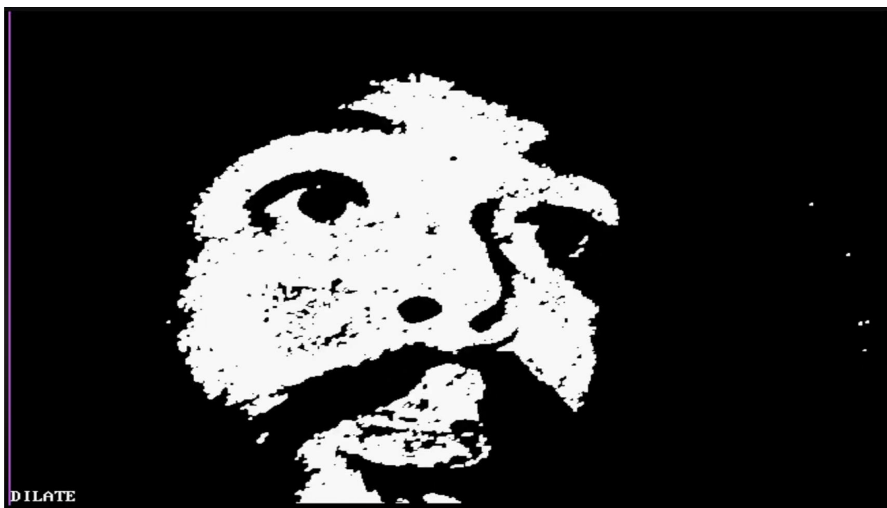
Figure 30:Dilation Filter Video Output
